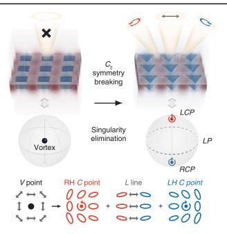
FIG. 1. Schematic view of how circularly polarized states (*C* points) spawn from a bound state in the continuum when in-plane inversion ( $C_2$ ) symmetry is broken. *C* points and lines of linearly polarized states (*L* lines) could be found near  $\Gamma$  point. The asymmetric field of the mode induces extra in-plane multipole moments. L(R)CP: left(right)-handed circular polarization; L(R)H: left(right)-handed.
