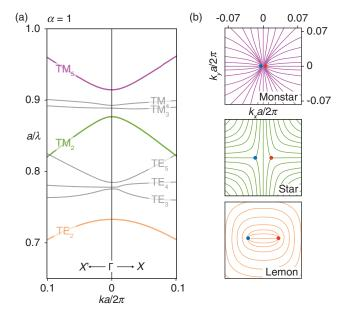
FIG. 3. (a) The band structures along  $\Gamma$ -X and  $\Gamma$ -X' near the  $\Gamma$  point. (b) Different configurations of polarization main axis near the  $\Gamma$  point on bands TE<sub>2</sub> (bottom, "lemon"), TM<sub>2</sub> (middle, "star"), TM<sub>5</sub> (top, "monstar") of the structure with  $\alpha = 1$ . The different colors correspond to the colored bands in (a).
