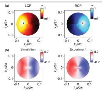
FIG. 5. (a) Experimental observation of the coverage on Poincaré sphere presented in the form of transmittance maps along the band  $TE_2$  in the visible frequency range. (b) Simulated and measured ellipticity maps of transmitted polarization states under p incidence on the same band as in (a).
